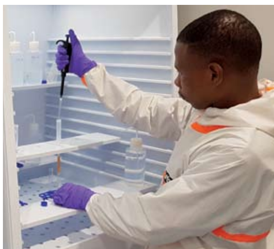
Masters student, Sibusiso Khonyana (from UJ), at work in the WIGL, collecting 1ml elute increments for the calibration of Be and Al chromatographic separation (photo courtesy of Tebogo Makhubela)
