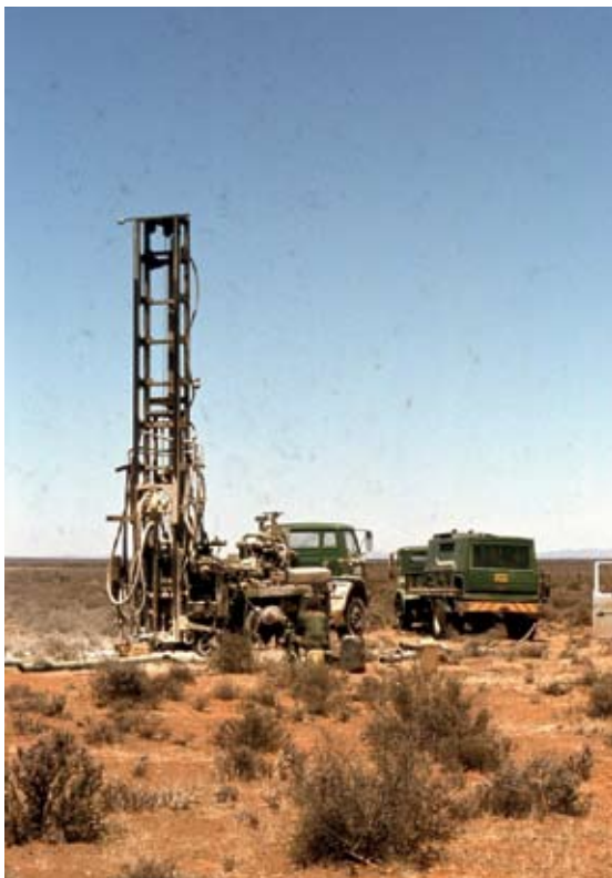
Conventional percussion drilling rig in action in the Karoo region during the height of uranium exploration in the late 1970s.
