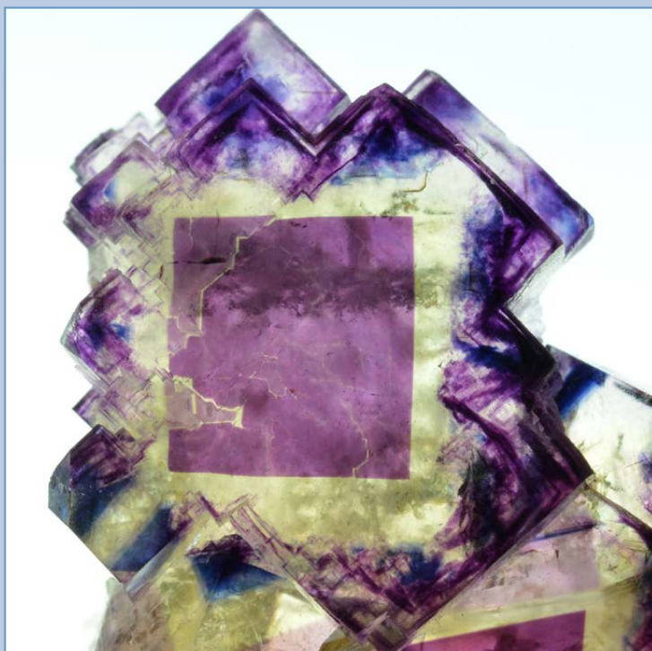
Internal colour zoning in fluorite from Okorusu mine, Namibia. Field of view is 3 cm.
